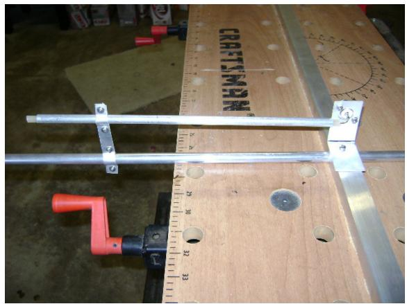
**Figure 7.** Gamma match assembly to boom installation. The view is looking towards the director.
